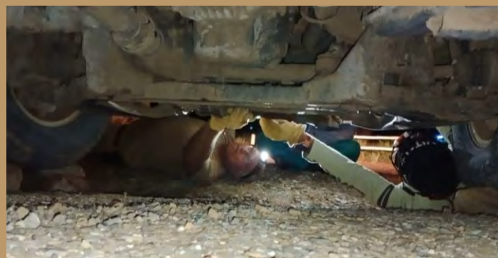
Figure 25: Arne and Alex securing the body plate back into place using cable ties during field repairs.
